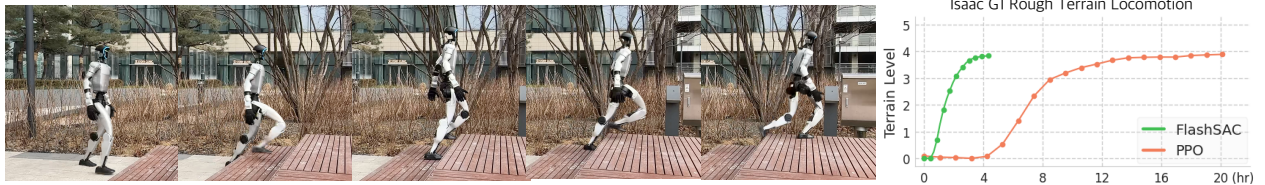
Figure 6 Sim-to-real Stair Climbing on Unitree G1. FLASHSAC achieves stable real-world stair climbing after only 4 hours of training on simulation, whereas PPO requires nearly 20 hours to reach the same capability.
